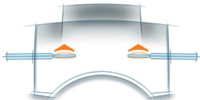
In case you have to reinsert the lenses: The flat part of the lens facing the eye and the curved part facing the display.
